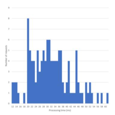
MEC-assisted position calculation time (Regular PC in the access network)
