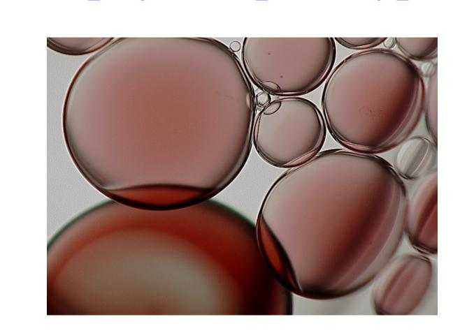
A physical prototype of the network are droplets containing reagents of photosensitive BZ reaction in the water phase. The droplets are surrounded by the oil phase containing lipids that stabilize them mechanically. Touching droplets communicate via diffusion of reaction activator (HBrO2) through the lipid bilayers.
